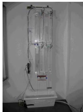
b) Coupled water tanks experimental setup
