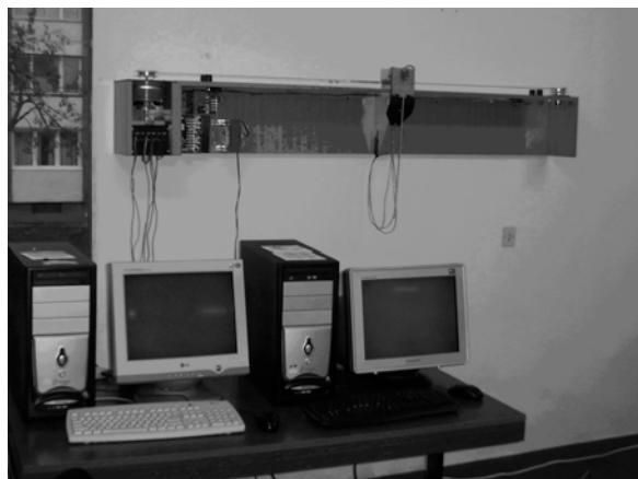
a) Inverted pendulum & crane set-up
